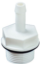
7WTFITT10 Ref. 680169 Threaded Barb fitting 3/4" BSP to 10mm To be used with fresh water tanks.
