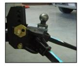
IT IS IMPERATIVE THAT ONLY A 50mm TOWBALL WHICH CANNOT UNWIND ITSELF BE USED WITH ANY AKS STABILISING COUPLING HEAD.
