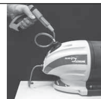
Diagram 1. Attaching the bleed gun to the actuator.
