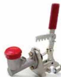
610943 Coupling Hydraulic Conversion With 3/4" Master Cylinder
