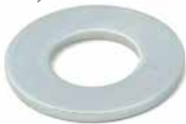
190015 Washer 25.9 I.D. x 53.6 O.D. x 3.9 Suits 1.5T, Parallel, 2T, 2.5T Machinings
