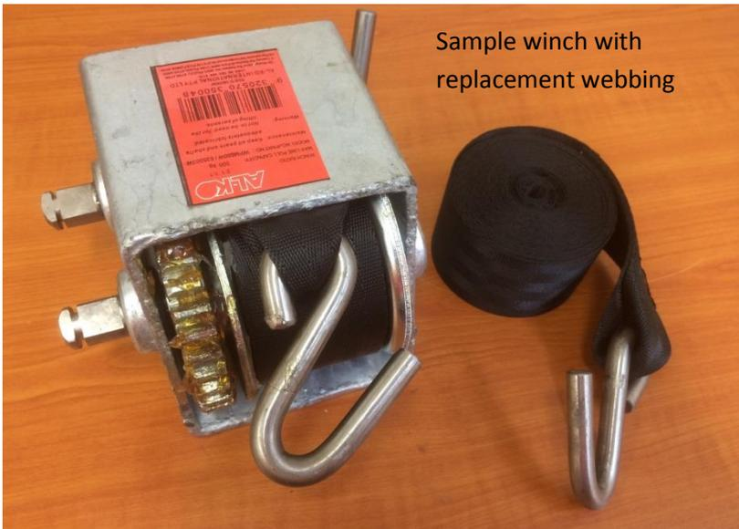
The first step is to fully unwind the winch webbing to expose the drum core and roll pin that holds the shaft in place.
