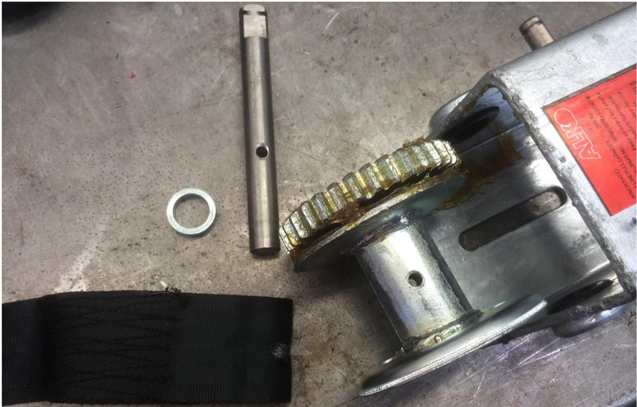
The parts after disassembly are shown above. The installation of the new webbing is simply the reverse of the disassembly, with the following points.
